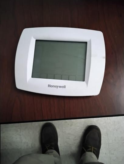
This T-stat has been damaged and will not move from 62 degrees and will need to be replaced. Asset 4043 Room 229 in the training bldg.
