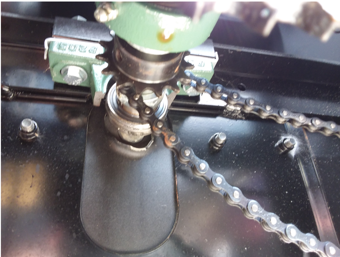
old broken pillow block bearing
