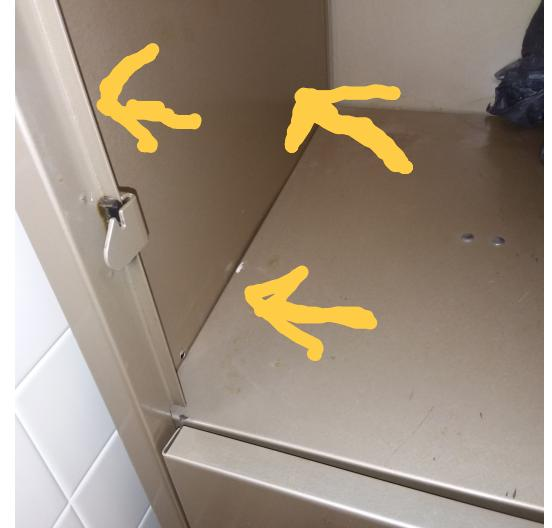
9 bolts on each side top to bottom, 27 nuts and bolts, both sides and back of locker coming off.
