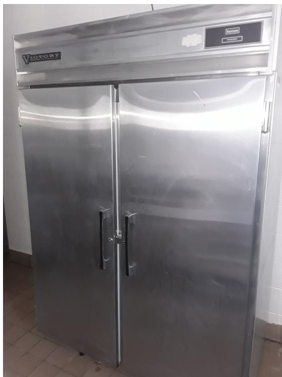
Asset 6788 & 6877 - Both are not working - Both have failed compressors and are tripping there breaker.
