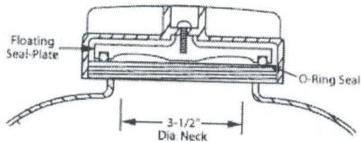
Cross dissection of the 1/4 buttress threaded cap assembly with self aligning floating seal plate between the neck of feeder and cap.
